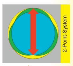
In the machining of bores, very often 3-jaw chuck or collet chucks are used. This has the consequence that the work pieces can be deformed. These polygon-deformations can significantly affect the quality, or even create scrap. An accurate measurement is only possible with 3-point tools, in which the probes are arranged at 120°. By changing the measurement position, the difference can be determined from the largest to the smallest diameter.
