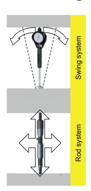
With swivel internal measuring instruments, trough commuting around the solid plunger, the turning point is determined. The minimum value can be recognized by a dial gauge, by the change of direction of the pointer. Usually, only a small measuring range is available. Proper handling requires feeling, usually 2 axes have to be coordinated manually.
