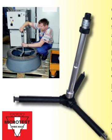
Our MICROTEST® system is the only one that can measure bore holes from Ø 400 mm to Ø 1150 mm precise and accurate.
