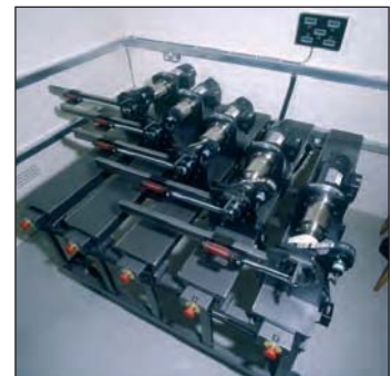
Norbar 5 station tester is used for durability and benchmark testing.
