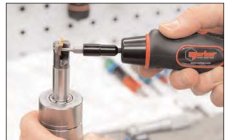
Bit holder can be removed and replaced with widely available screwdriver blades.
