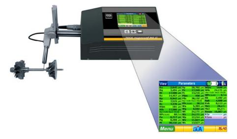
More than very accurate а measuring system, the 90G allows with the touch screen various calculations and analysis of graphics and curves. The complete list of parameters with background that changes according to tolerances. All graphics, roughness, primary profil and wawiness are displayed and use zoom function for more details, for example on scratch zone. specific Distribution curves with calculated values, directly on the instrument.
